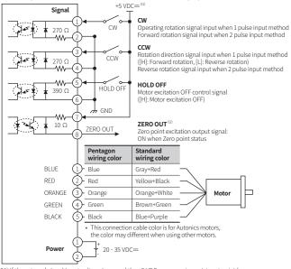
01) If the external signal input voltage is exceed the +5 VDC=, connect a resistor at outside. 02) ZERO OUT is only available for MD5-HD14-3Xand option.
